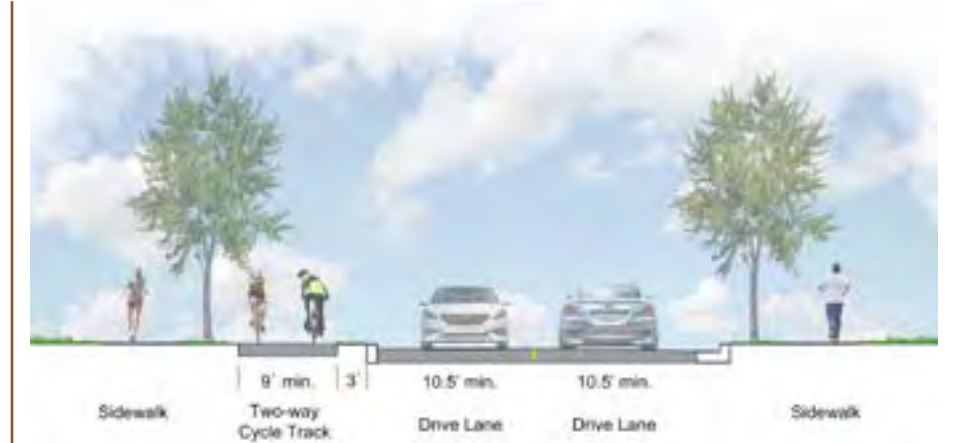
Raised Two-way Cycle Track Typical Section
